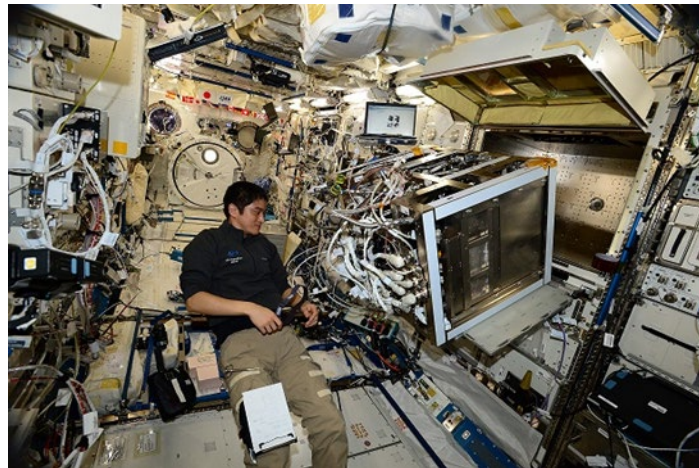
Figure1 Electrostatic Levitation Furnace on the International Space Station
